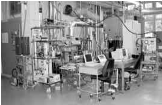
Figure 3: Test equipment with the under stoker wood furnace, samplin in the flue gas, and particle measurement systems with data acquisition.
