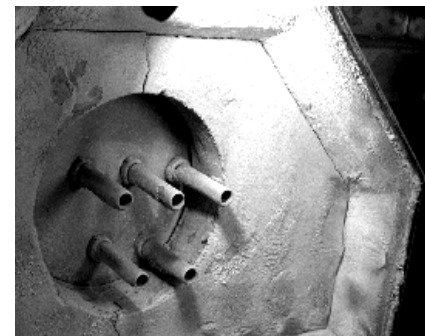
Figure 4: Test equipment for pneumatic cleaning of heat exchanger tubes with pressurized air [15,16].
